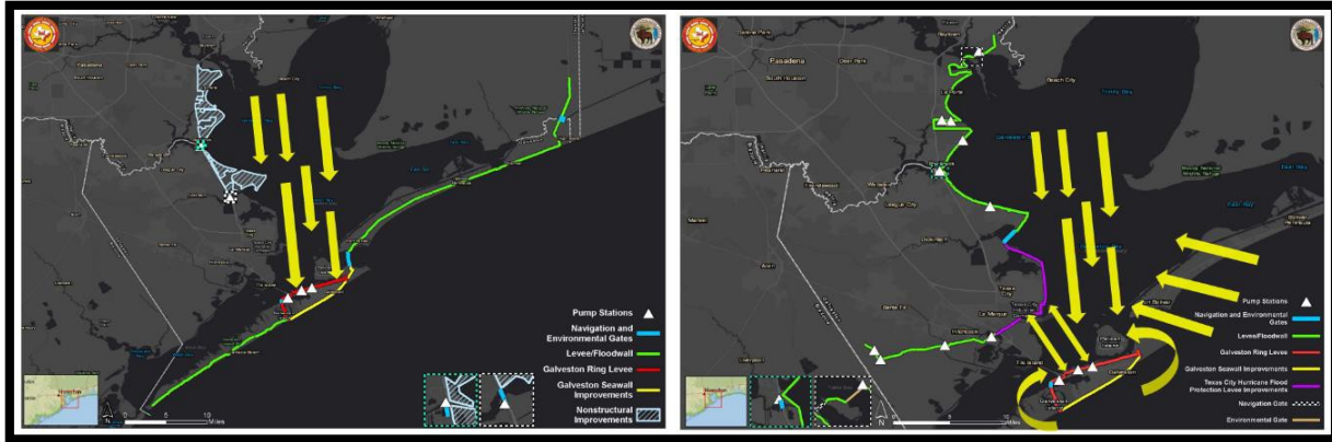
Figure 43 - Surge Forces on Galveston Ring Levee
