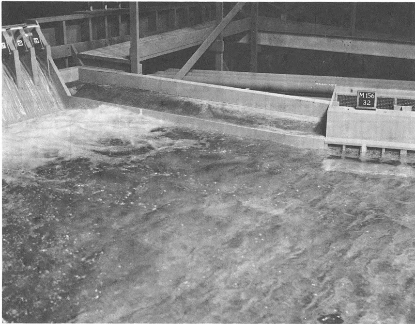
Spillway discharge 440,000 cfs.
