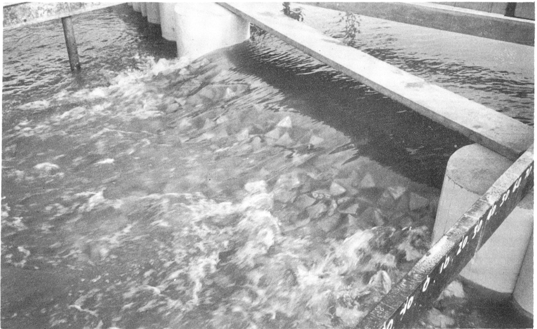
Fig. 29 - Construction Model - Fourth Experiment Water Surface with 1722 tetrahedrons
