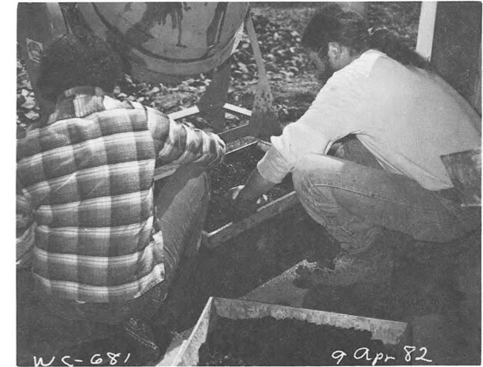
SIEVING AGGREGATE FOR MIXER PROFICIENCY TESTS.
