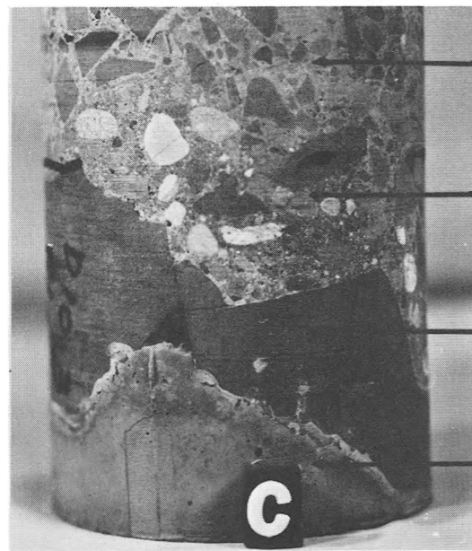
SIX-INCH CORE THROUGH THE RCC AND BEDDING INTO THE FOUNDATION ROCK. SAMPLE PREPARED FOR SHEAR TEST.
