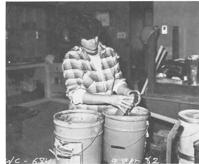
WASHING COARSE AGGREGATE FOR MIXER PROFICIENCY TESTS.
