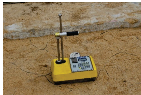
(b) Nuclear moisture and density gauge test.
