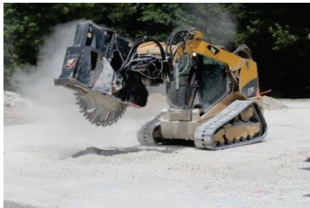
(a) Cutting with SW60 attachment.
