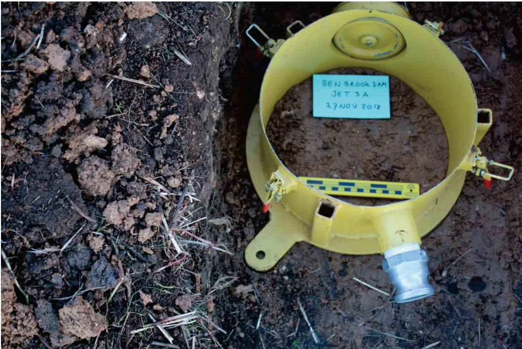
Figure 6. The JET steel chamber driven to the soil surface to keep the soil surface under water during the test.
