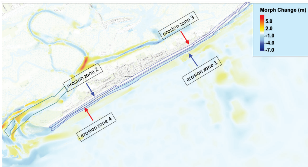
Figure 4-58. Morphology changes for the base case nearshore in front of Folly Beach in 2018. Warmer colors represent sediment accretion (delineated by red lines) and cooler colors sediment erosion (delineated by blue lines).
