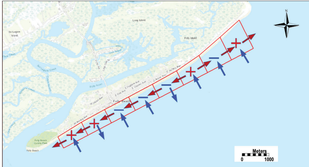
Figure 4-59. The calculated total sediment transport directions across polygon lines. The positive sign indicates bed volume gain and the negative the volume loss within the corresponding polygon area.
