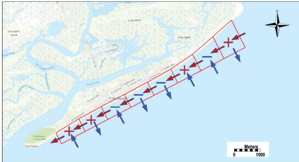
Figure 4-31. The calculated total sediment transport directions across polygon lines. The positive sign indicates bed volume gain, and the negative sign indicates volume loss within the corresponding polygon area.
