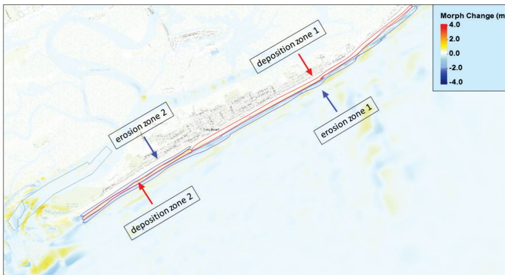
Figure 4-24. Morphology changes for the base case nearshore in front of Folly Beach from 18 to 25 September 1989. Warmer colors represent sediment accretion (delineated by red lines), and cooler colors sediment erosion (delineated by blue lines).
