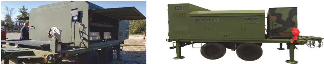
Figure 21. Enerdel 40 kWh lithium-ion energy storage system.
