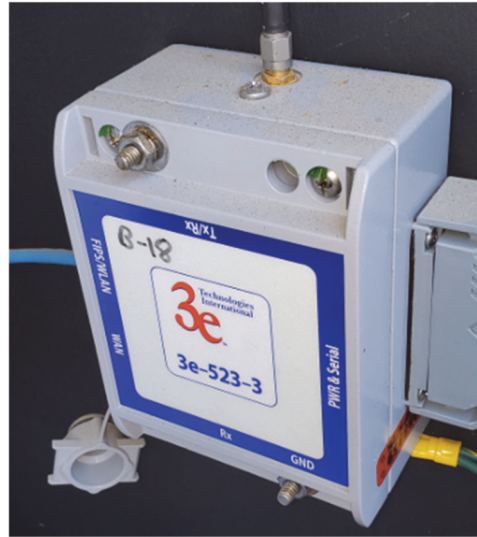
Figure 24. DMMS wireless access point.
