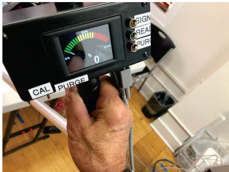
Figure 11. Successful reading of nitroglycerine after probing for explosive compounds.
