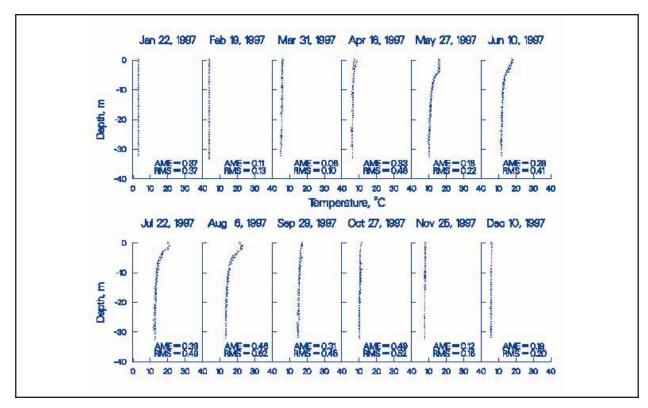
Figure 28. 1997 Bull Run Reservoir 2 computed versus observed temperatures
