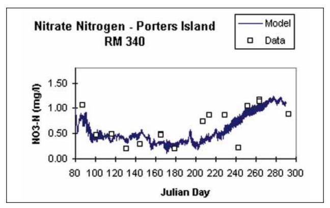
Figure 23. Computed versus observed nitrate/nitrite
