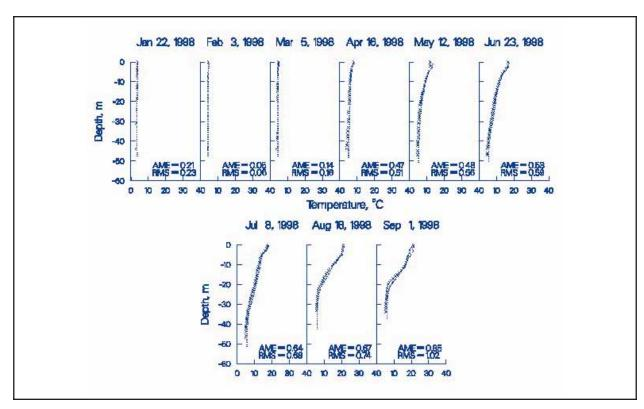
Figure 27. 1998 Bull Run Reservoir 1 computed versus observed temperatures
