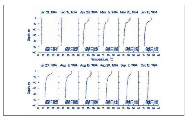
Figure 5. 1994 RBR computed versus observed temperature
