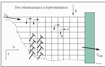
Figure 1. Typical CE-QUAL-W2, Version 2 model grid
