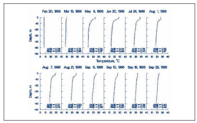
Figure 6. 1996 RBR computed versus observed temperature
