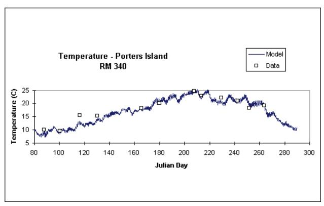
Figure 20. Computed versus observed temperatures
