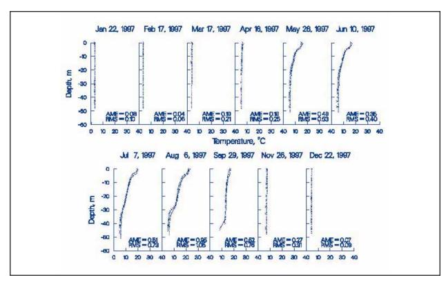
Figure 26. 1997 Bull Run Reservoir 1 computed versus observed temperatures
