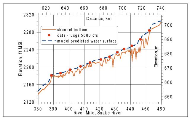
Figure 19. Comparison of model predictions and data of water surface along a portion of the Lower Snake River at a flow of 5600 cfs
