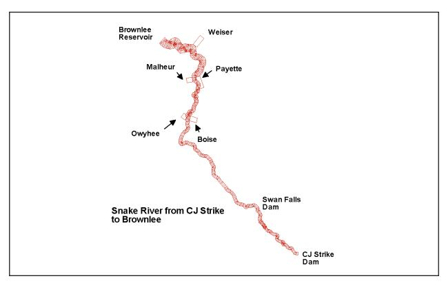
Figure 18. Lower Snake River model segmentation
