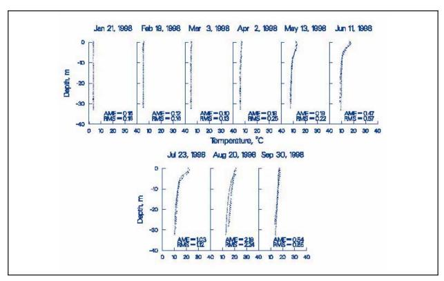
Figure 29. 1998 Bull Run Reservoir 2 computed versus observed temperatures
