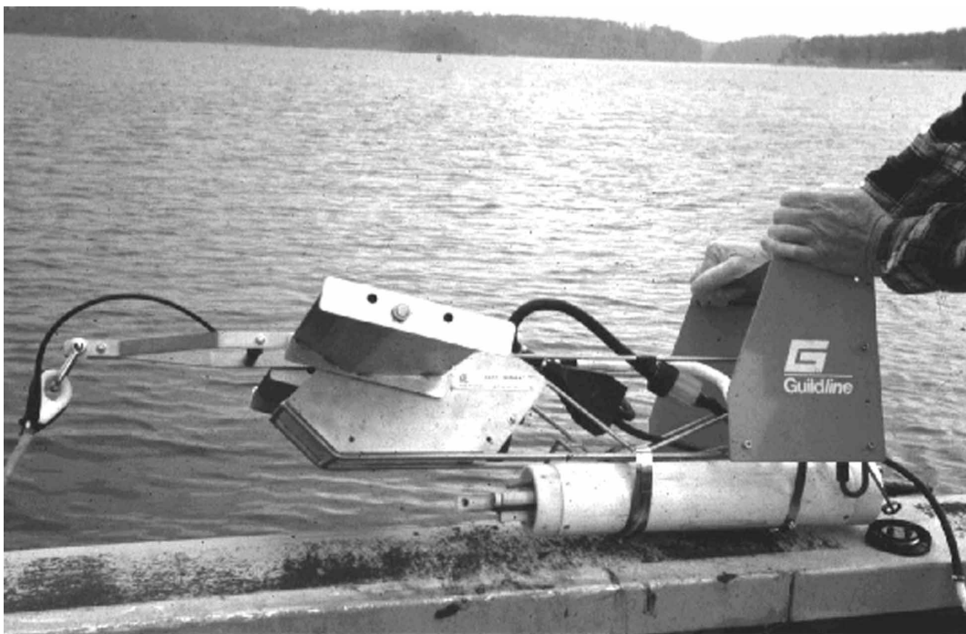
Figure 1. Guildline Minibat with Hydrolab water quality sonde attached
