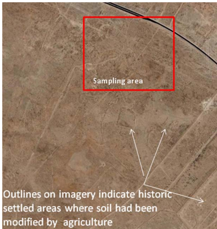
Figure 2. Image from a middle-eastern desert showing historic areas of AM soil (white arrows). EM and UM soils appear within the soil-sampling area indicated in the figure, which includes a paved highway with adjacent soil berms (EM soil), lightly graded low-volume roads (EM), and evidence of other human activity (UM).
