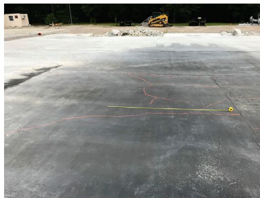
(f) Low-severity shattered slab in Quadrant #1 at 1,664 passes
