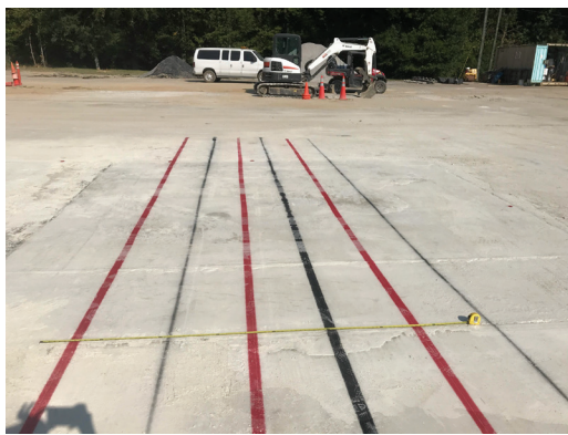
(a) No visible cracking on repair (Quadrant #3) at 0 passes
