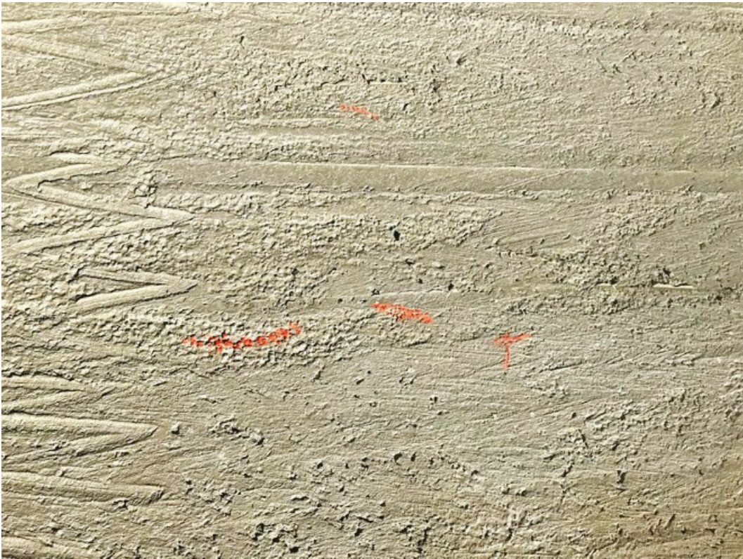
Figure 41. Spalling on parent slab in the trafficking area at 224 passes.
