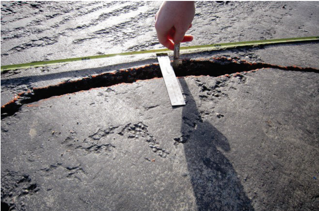
Figure 38. Parent slabs adjacent to the repair started to spall after 1,680 passes.
