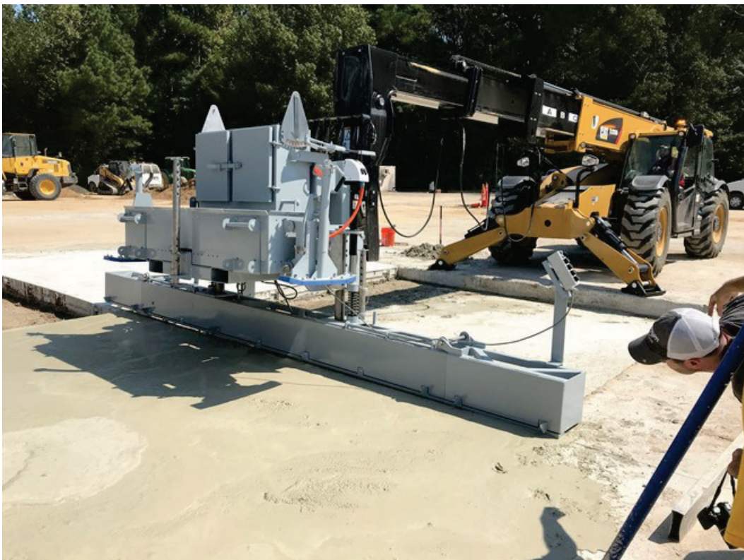
Figure 30. Modified prototype screed, RADR Screed.
