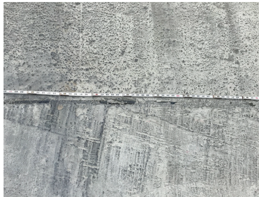
(b) Paste at joint starting to break up at 112 passes
