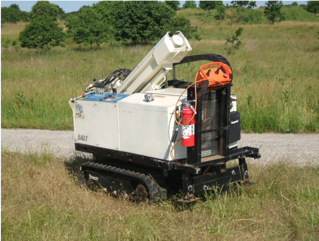
Figure 2. Track-mounted GeoProbe drill rig.
