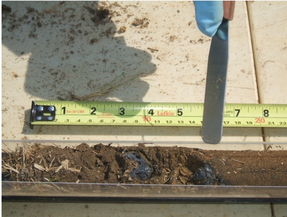
Figure 7. Example of metal slag fill within a cut acetate sleeve from the Soil Sampler.
