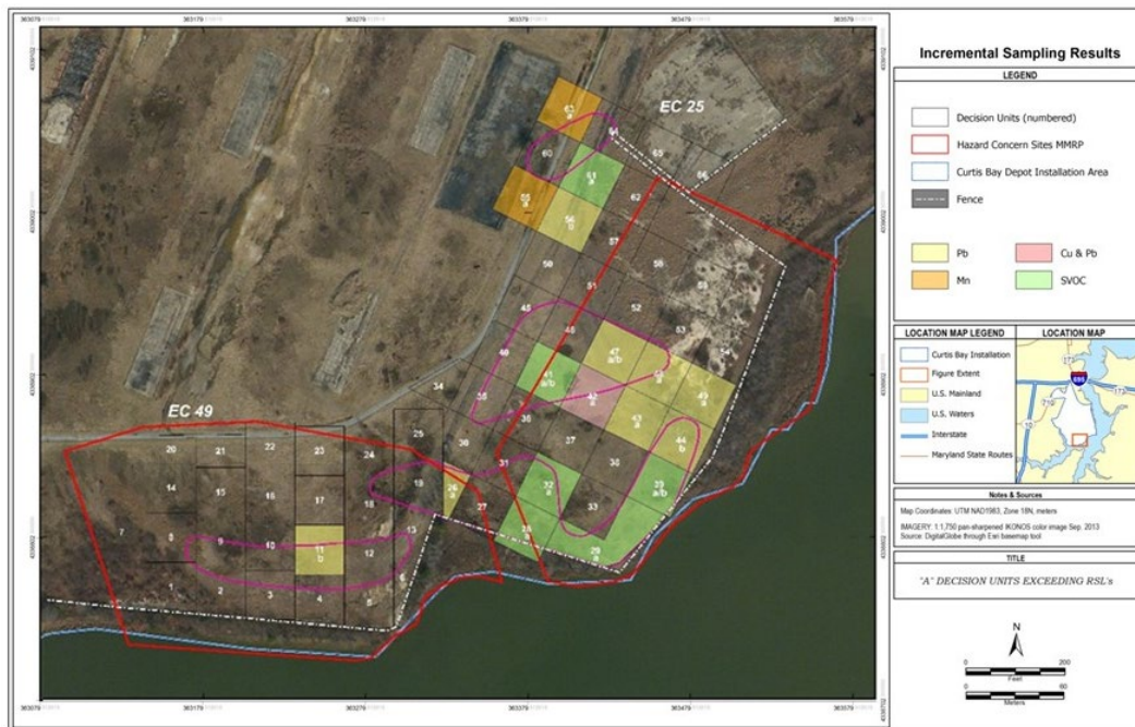
Figure 11. Revised ISM remediation zone compared to the original grab sampling method remediation zone.
