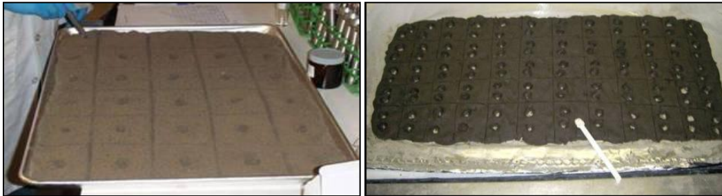
Figure 10. Examples of the multi-increment sampling approach used in the laboratory (a.k.a. the two-dimensional Japanese Slab Cake method) to prepare the subsample for digestion and extraction.
