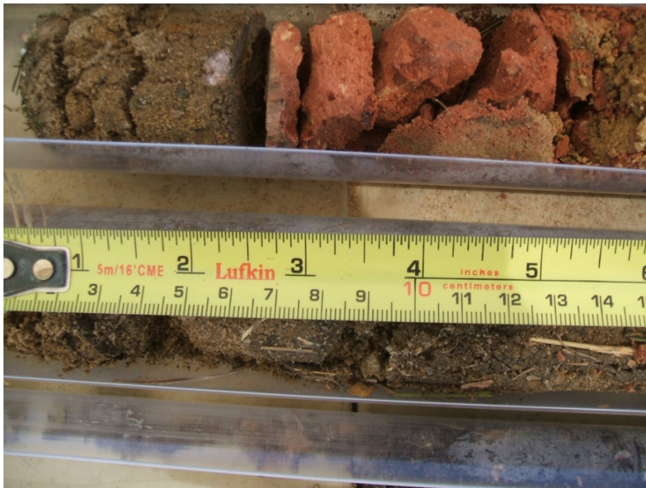
Figure 6. Example of red brick fill material.
