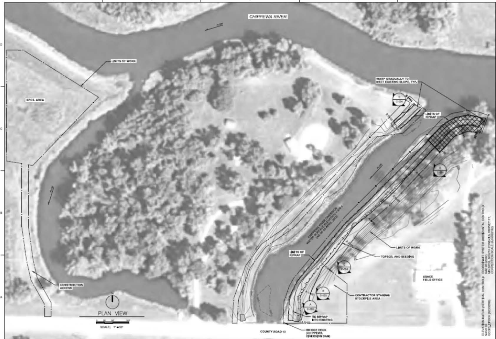
Figure 8. Map of the proposed bank stabilization for the Chippewa River Diversion Dam approach channel.
