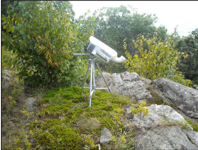
Figure 6. Anabat II acoustic detector field mounted for passive sampling.
