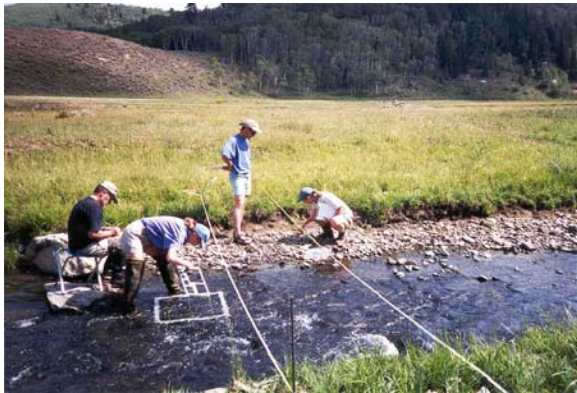
Figure 3. Researchers on the left performing a Wolman Pebble Count using a gravelometer and sampling grid.
