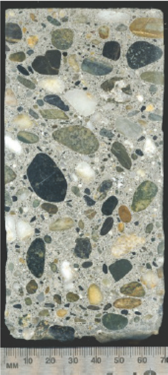
Figure C-11. Sample 11, hardened air-void analysis (9.57%).
