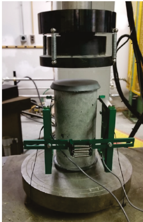
Figure 5. Modulus of elasticity test setup with extensometer.
