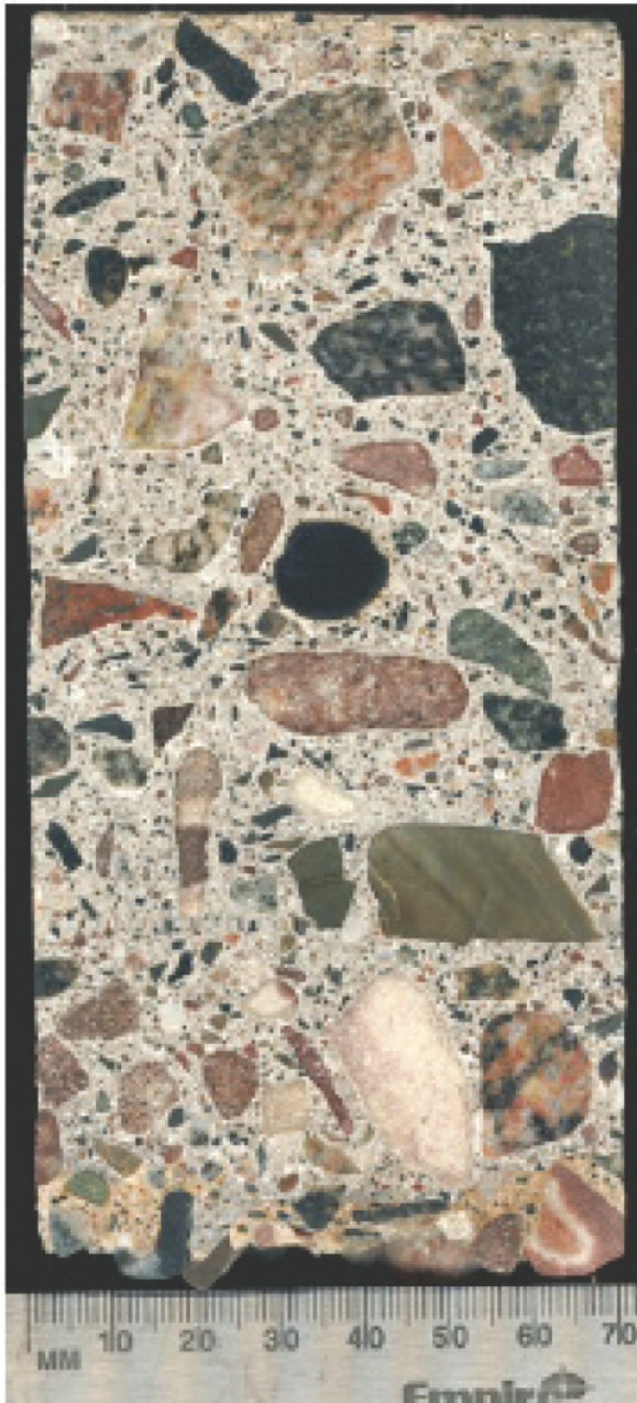
Figure C-1. Sample 1, hardened air-void analysis (4.59%).
