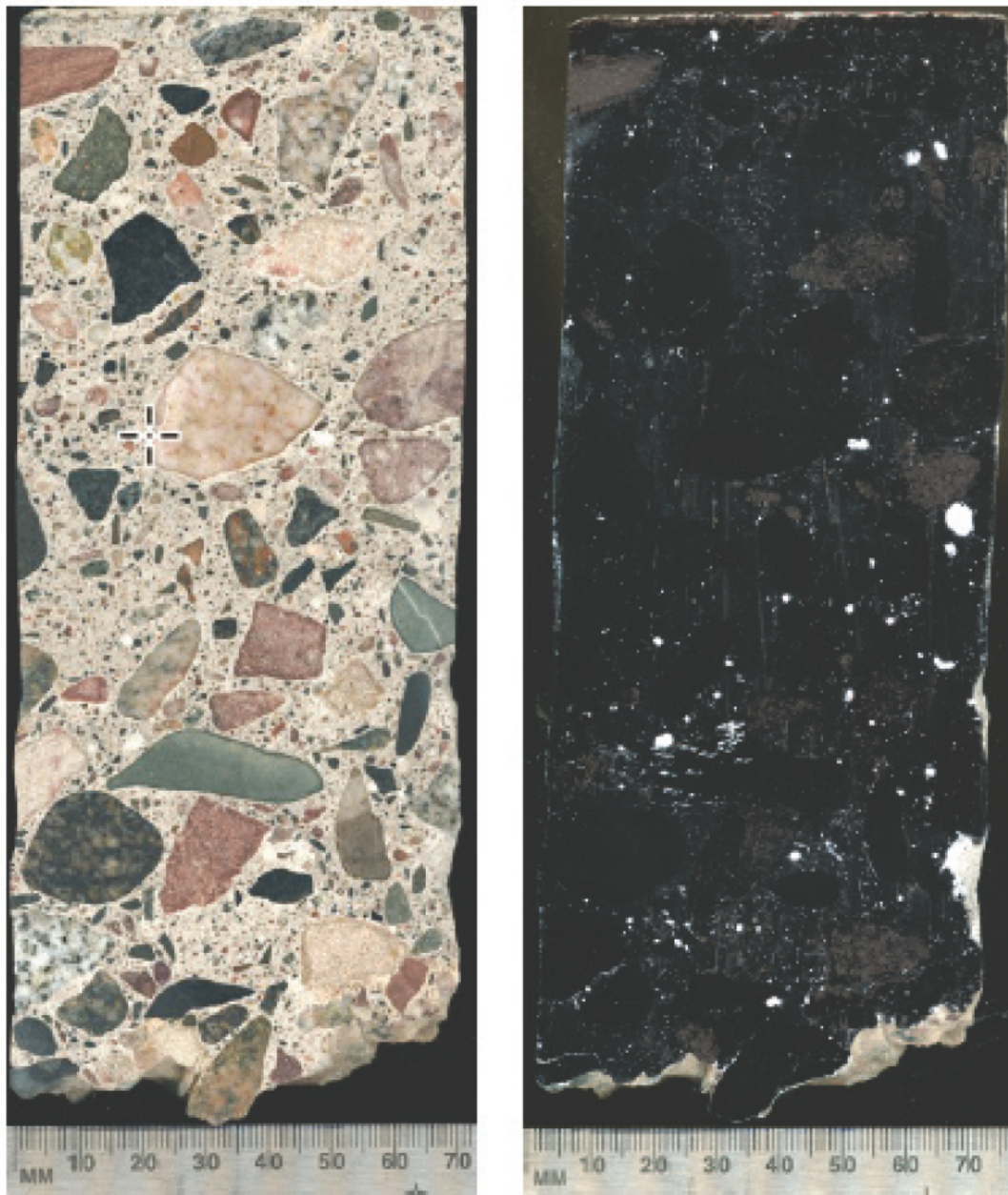
Figure C-2. Sample 2, hardened air-void analysis (3.87%).
