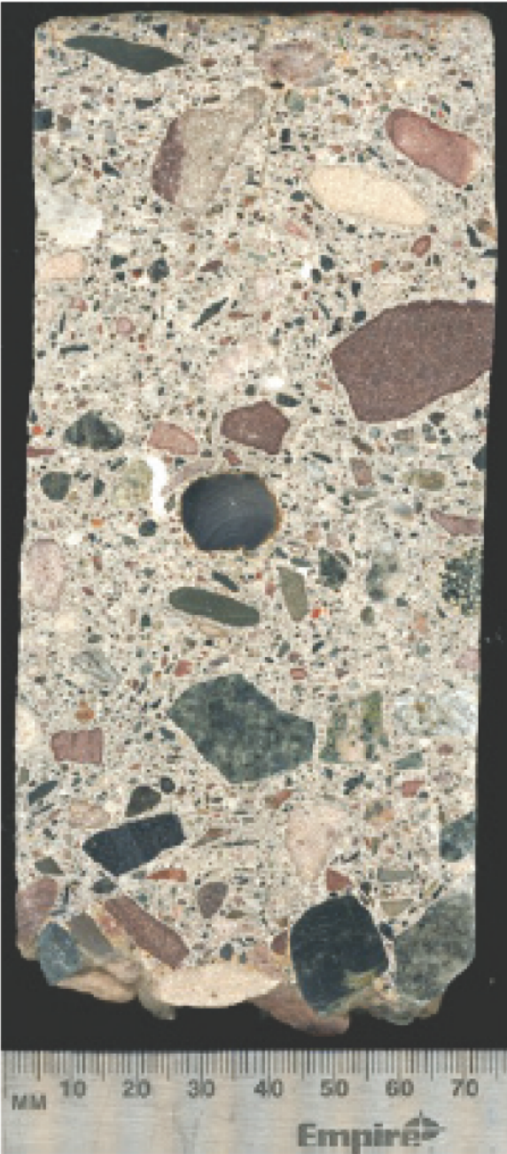
Figure C-3. Sample 3, hardened air-void analysis (9.47%).
