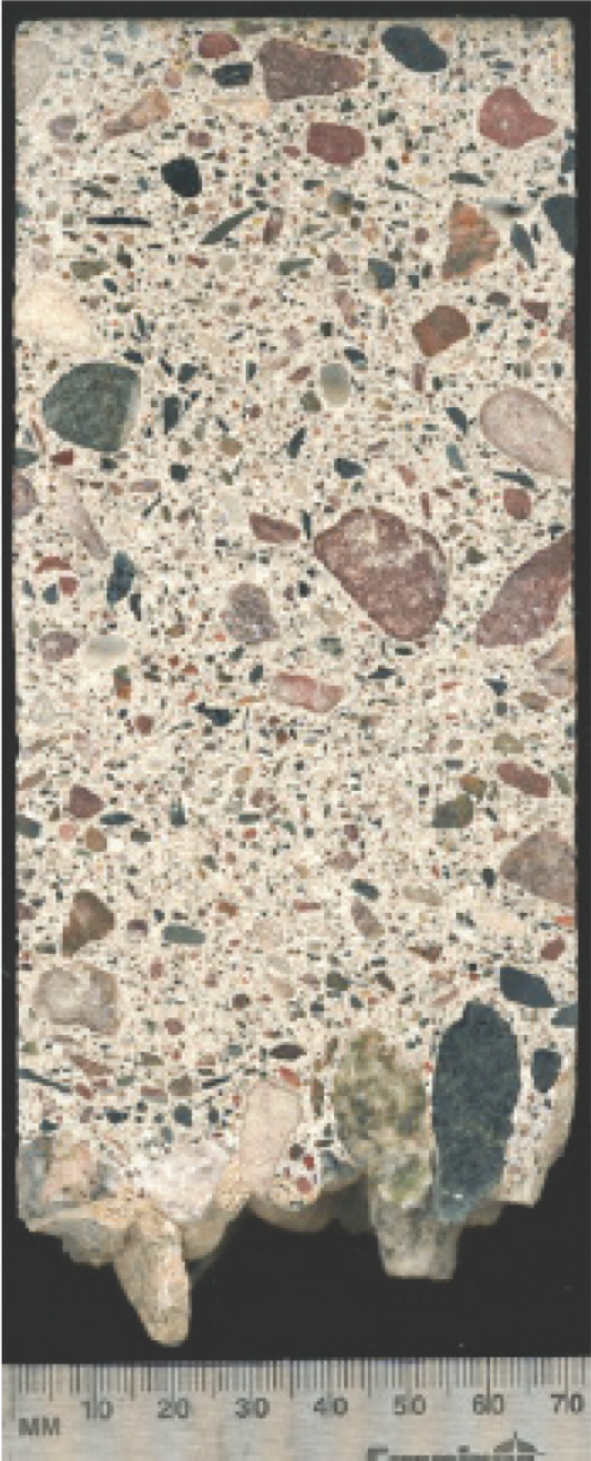
Figure C-6. Sample 6, hardened air-void analysis (10.6%).
