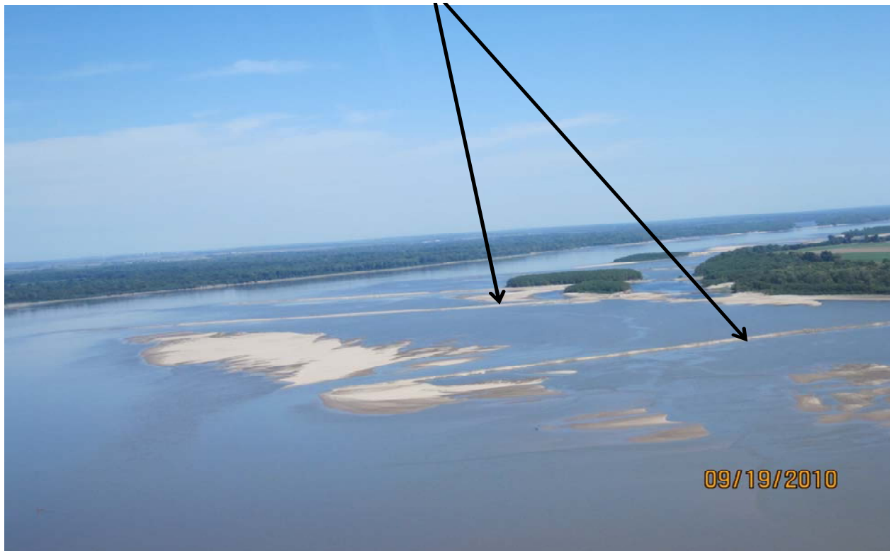
b. Closing dikes in a secondary channel of the Lower Mississippi River.
