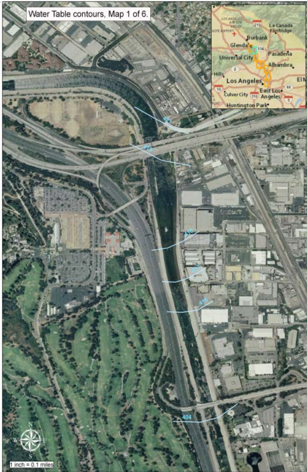
Contours shown are the approximate elevation of groundwater encountered.
