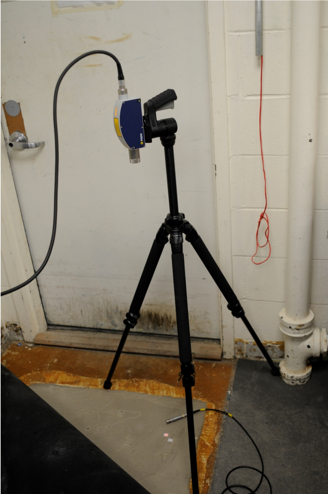
Figure 3. LDV sensor head mounted on the tripod and the microphone placed on floor.
