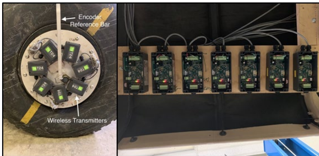
Figure 4. A wheel force transducer unit installed on one of the wheels of the HMMWV with transmitters and the encoder reference bar ( left ), and one of four receiver units installed inside the HMMWV ( right ).
