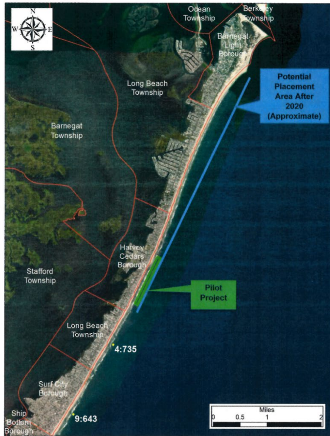
Figure 3: Beneficial Use of Dredged Material from the Maintenance of Barnegat Inlet, including the location of the pilot project, the additional nearshore area for future placement and the location of two shipwreck sites
