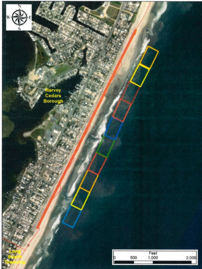
Figure 2. Close up of one-mile nearshore berm sand placement cells, approximately 500 ft x 300 ft each.
