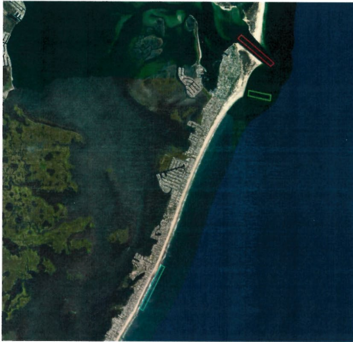
Figure 1. The red area is the existing Barnegat Inlet Federal Navigation Channel (sand source). The green area indicates one of the approved sand placement areas for the authorized Coastal Storm Management Project (LSI). The light blue rectangle is the proposed one-mile long nearshore beneficial use placement area adjacent to Harvey Cedars.
