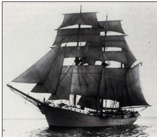
Figure 4. A rendering of a typical bark, in this case the German vessel Niobe (as presented in Naval Institute Press 1981).
