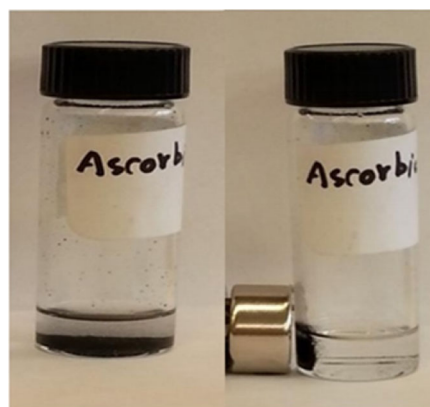
Fig. 4 Magnetic effects appeared after a permanent magnet was applied to separate the nanocarbons from water solution
