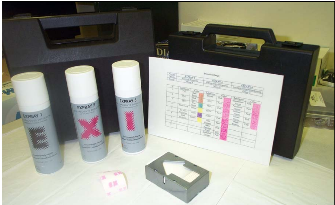
Figure 1. Expray Explosives Detection Kit.
