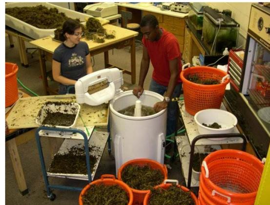
Figure 1. Wringer washing machine setup for processing small batches of seed-bearing plant stems.
