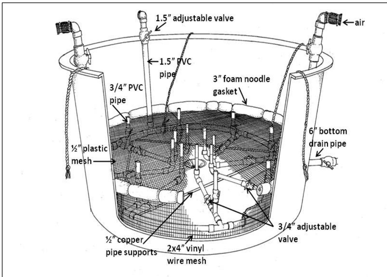
Figure 3. Schematic of turbulator design showing sizes and major component parts.
