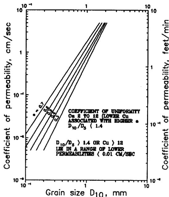
Figure 2. Permeability of sands and sand-gravel mixtures from void ratio and gradation data (After NAVFAC DM-7.1).  $e$  = void ratio;  $C_u$  = coefficient of uniformity,  $D_{80}/D_{10}$
