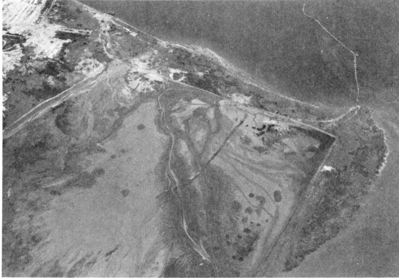
Fig. 20. View of McDuffie Island disposal area during disposal operations. Prominent channelized flow extends from dredge discharge point in upper center to sluice, off picture in lower center (Mobile District)
