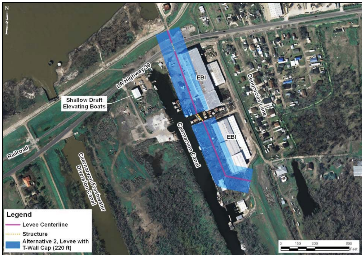
Figure 9. Alternative 2 - Realignment of Caernarvon Floodwall to Immediate Western Side of EBI Property
