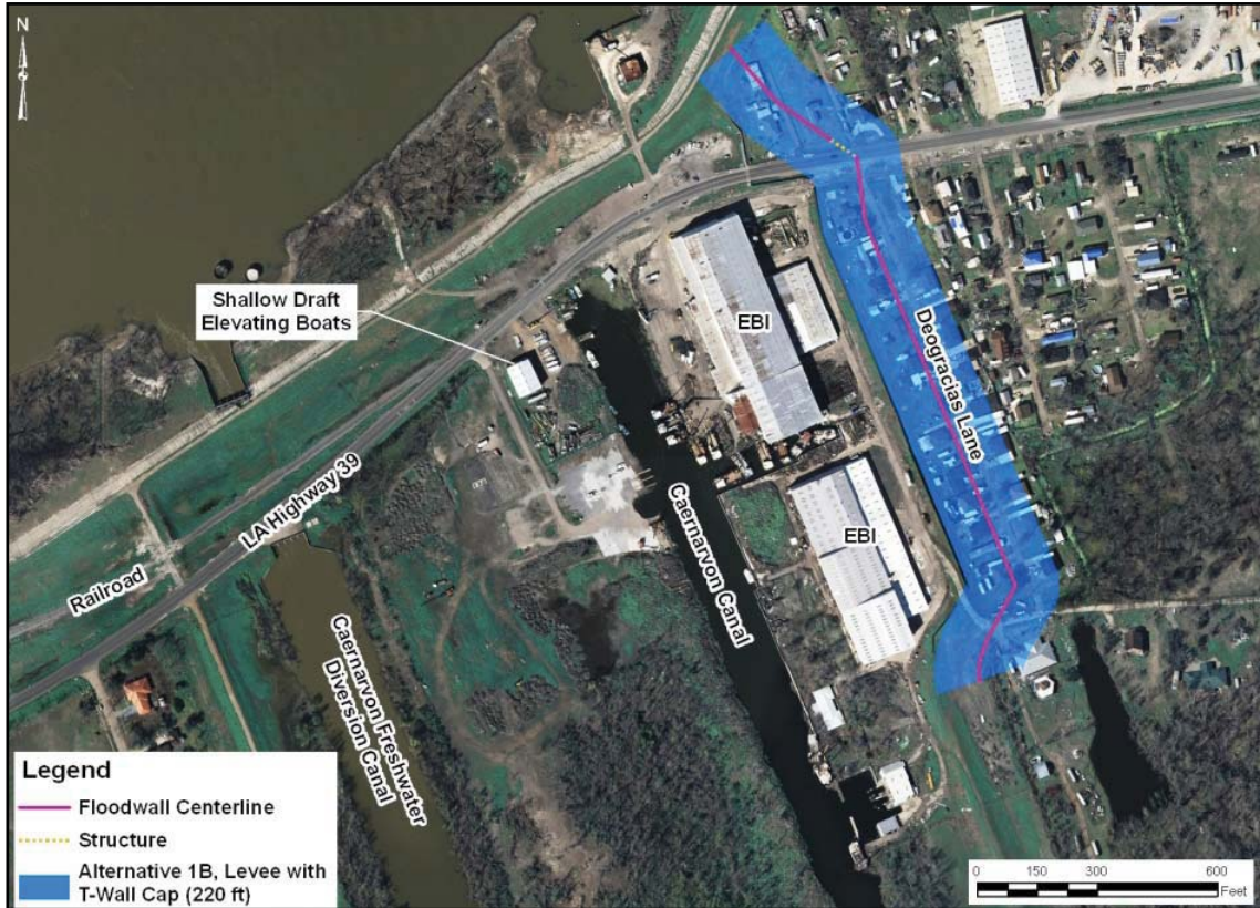
Figure 8. Alternative 1b – Modification or Replacement of Existing Flood Gates and Construction of a Levee with T-Wall Cap (Current Alignment, Slight Protected-Side Shift)
