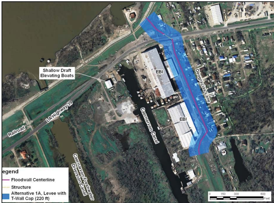
Figure 7. Alternative 1a - Modification or Replacement of Existing Floodgates and Construction of a Levee with T-Wall Cap (Current Alignment)
