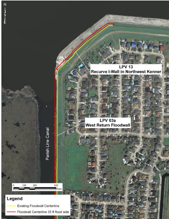
Figure 3a. LPV 13 and LPV 03a (northern portion) - Existing and Proposed Floodwall Alignment
