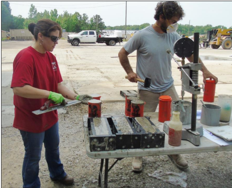
Figure 22. Field specimen preparation for compressive and flexural strength.
