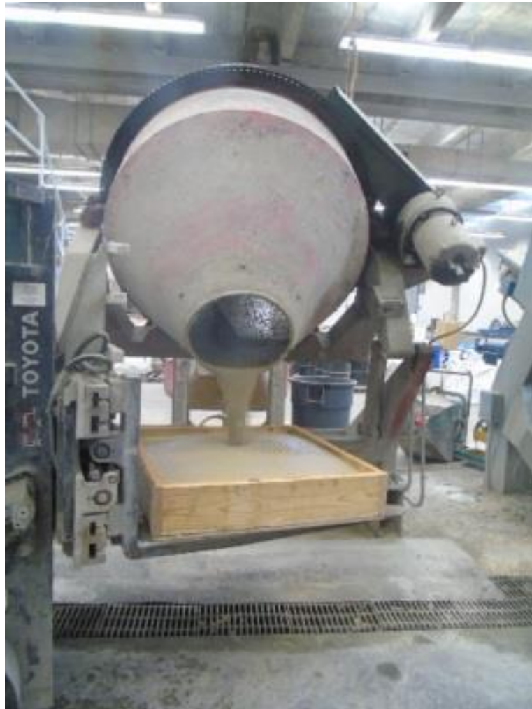
Figure 9. Displacement of MPC designed concrete into slab form.
