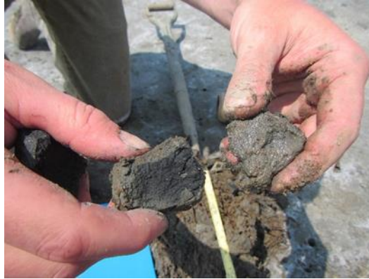
Figure 5. Dark soil coatings (soil on left) from iron sulfide soil materials at Avalon, then oxidized with 3% hydrogen peroxide (soil on right) resulting in removal of dark soil coating and revealing of the underlying grey soil matrix color.
