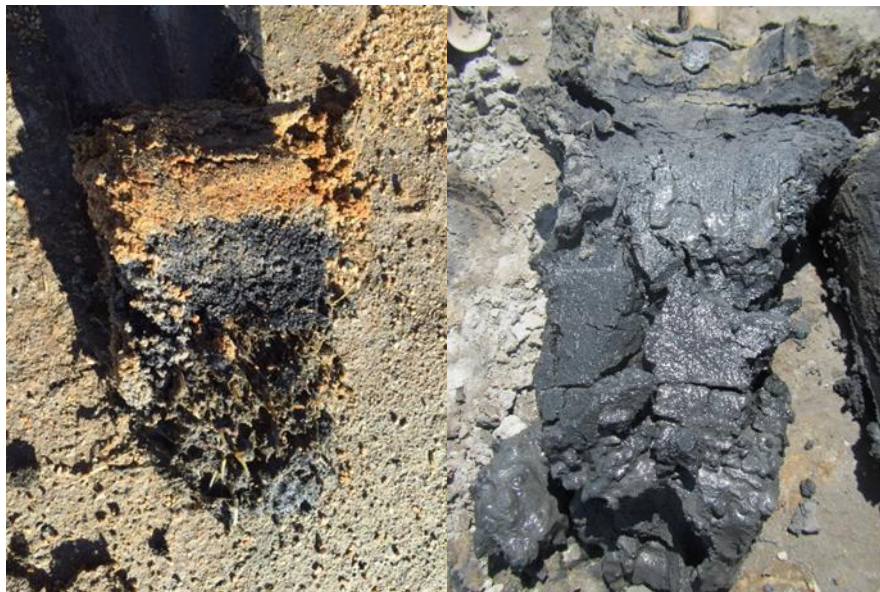
Figure 4. Narrow River (left) soil sample displaying black iron sulfide materials at the contact point between placed upland sands and the underlying marsh soils; Avalon (right) soil sample displaying extensive iron sulfides coating with recently placed dredged materials.
