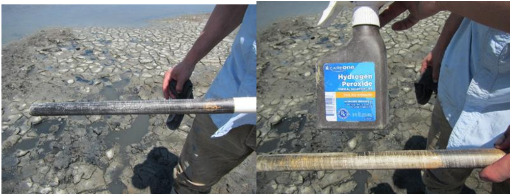
Figure 6. When present, free sulfides precipitate on the surface of Indicator of Reduction in Soils (IRIS) tubes within one hour of installation, resulting in the formation of a black coating (left). Removal of black coating on the IRIS tube by hydrogen peroxide oxidation (right).
