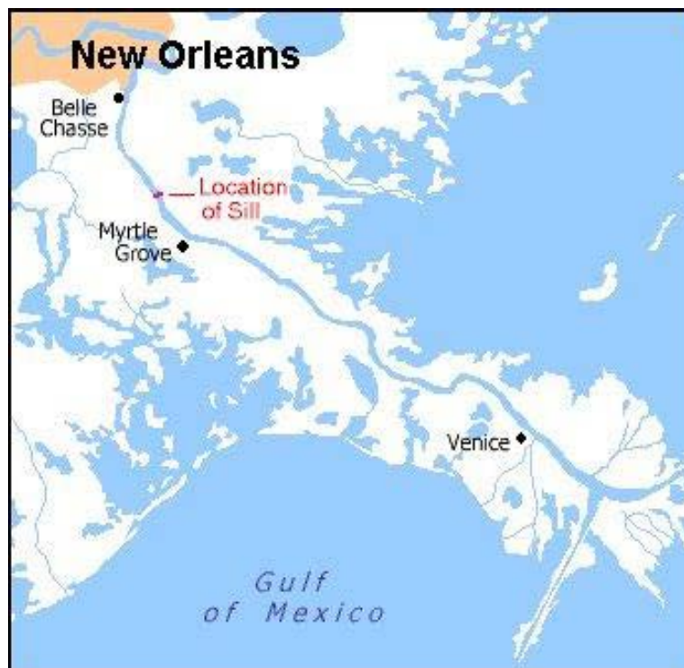
Figure 2-12 Location of emergency saltwater barrier sill south of Belle Chasse, LA
