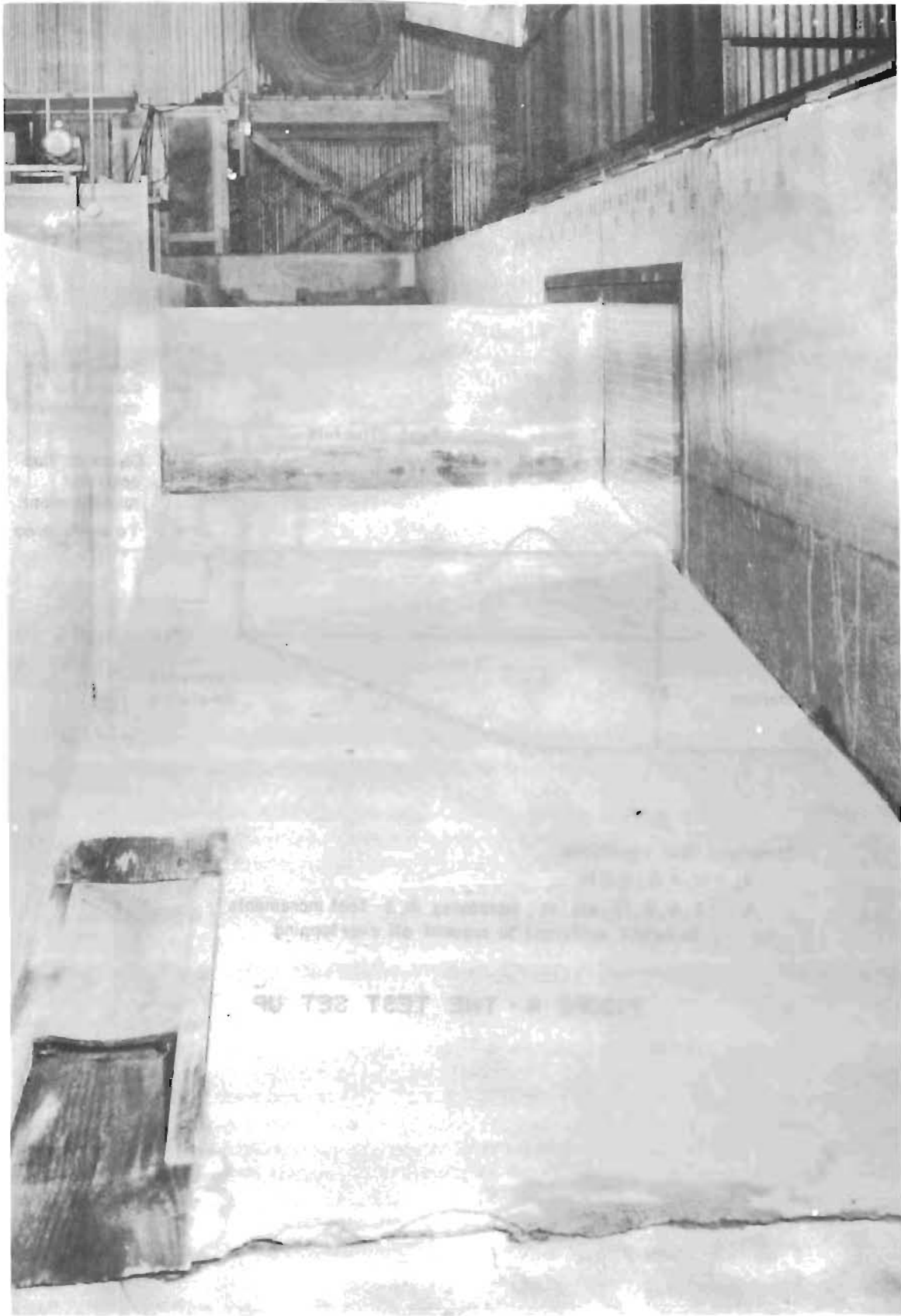
FIGURE 3. BEACH SLOPE AND VERTICAL WALL TEST SECTION
