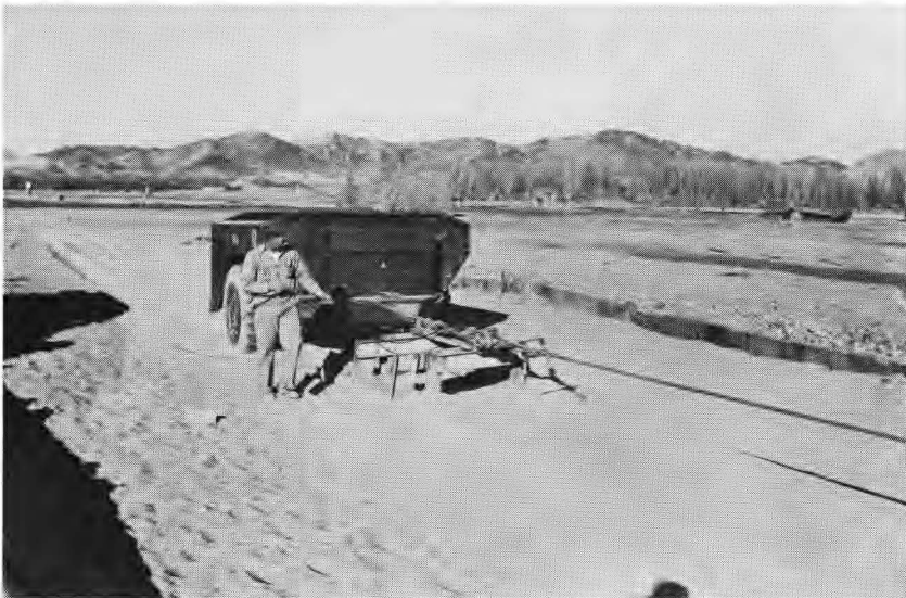
M21 loaded with 8,000 lb, tire pressure 30 psi, on the 2d pass in dry concrete sand. Test 12
