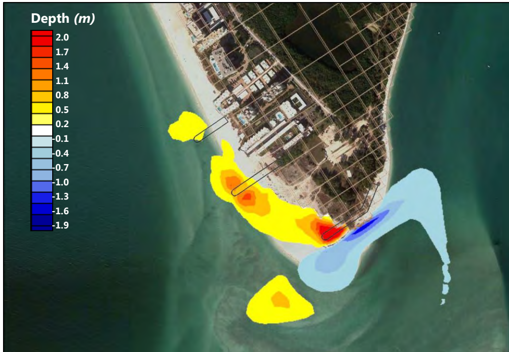
Figure 96: Groins without nourishment; Ending morphology difference for six month run 2004 = (groins were in place with no beach nourishment) – (no groins and no beach nourishment)
