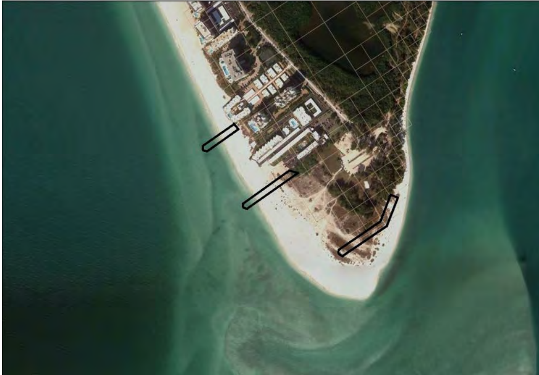
Figure 95: Plan view of groins; Groin design is from the 2004 Feasibility Report, 2013 Shoreline at Lido Key
