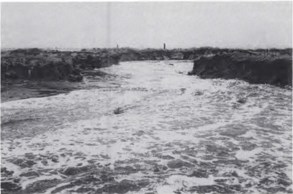
Photo 2. Initial breach formation, looking landward, 10 December 1993
