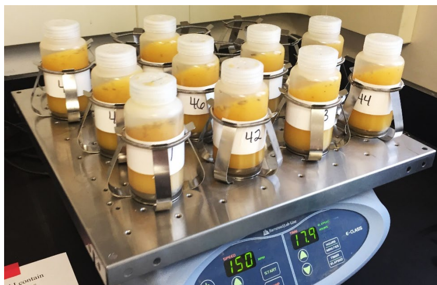
Figure 1. Batch-reaction shaker-table setup, showing reactions 41–50 (iron amendment).
