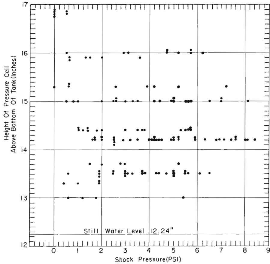
FIGURE 7 COMPARISON OF VERTICAL POSITION OF PRESSURE CELLS WITH SHOCK PRESSURES
