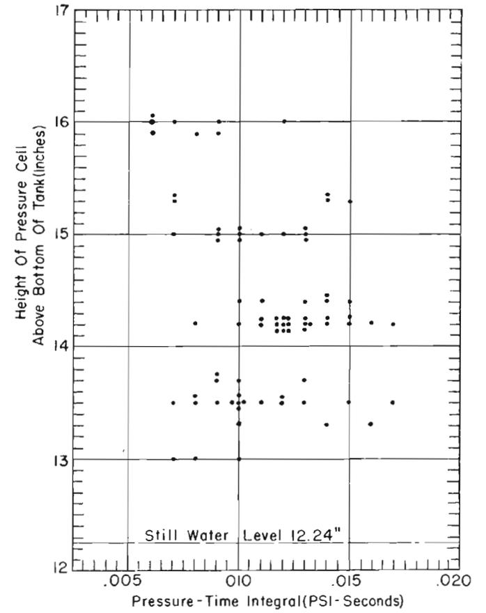
FIGURE 8 COMPARISON OF VERTICAL POSITION OF PRESSURE CELLS WITH PRESSURE TIME INTEGRALS
