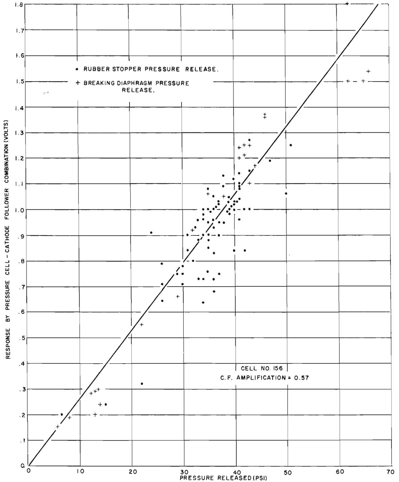
FIGURE 3 CALIBRATION OF PRESSURE CELL WITH CATHODE FOLLOWER
