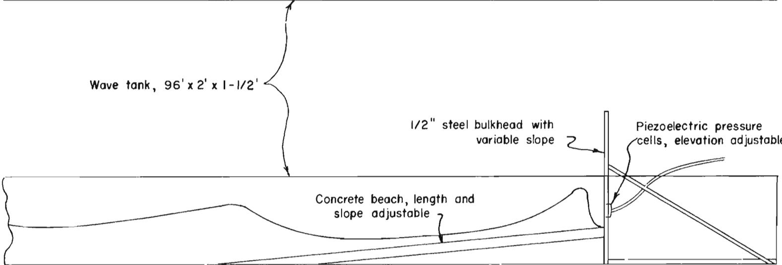
FIGURE I DIAGRAM OF WAVE TANK
