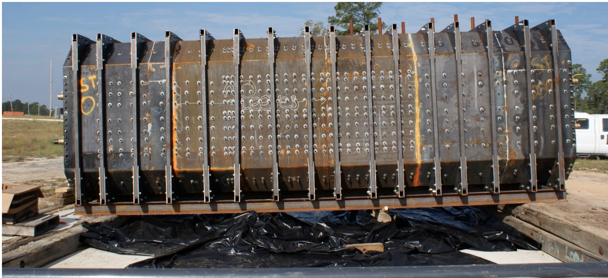
Figure 5. Inclined 7 ksi steel form.
