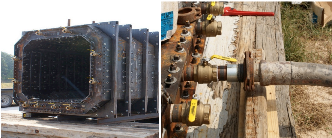
Figure 6. Ball valve arrangement (left) and ball valve connection (right).
