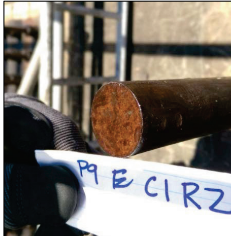
Figure 5. Typical rod without corrosion.
