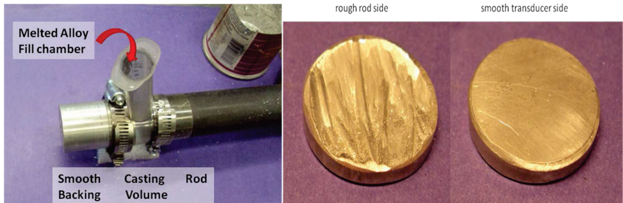
Figure 8. Trunnion rod end casting assembly and sample casting.
