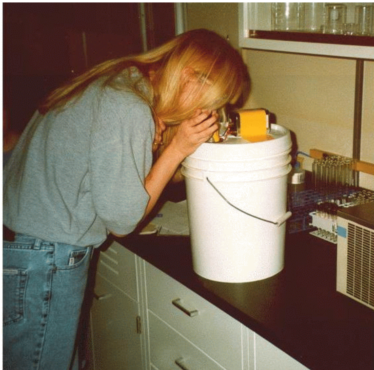
Figure G4. Panelist performing odor detection evaluation
