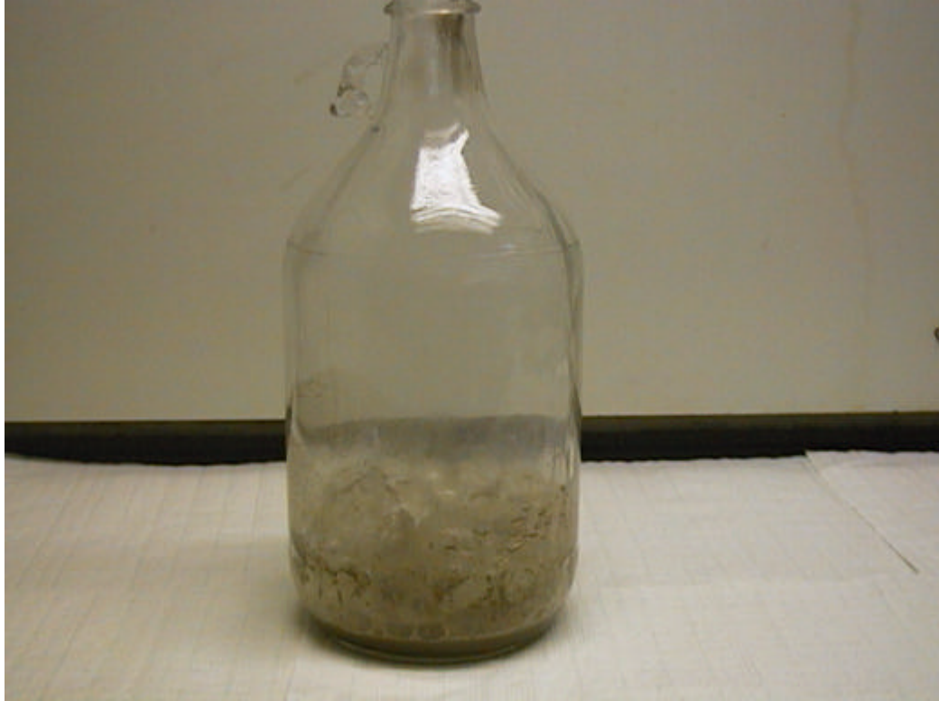
Figure C3. Oxidation of oven-dry sediment with hydrogen peroxide
