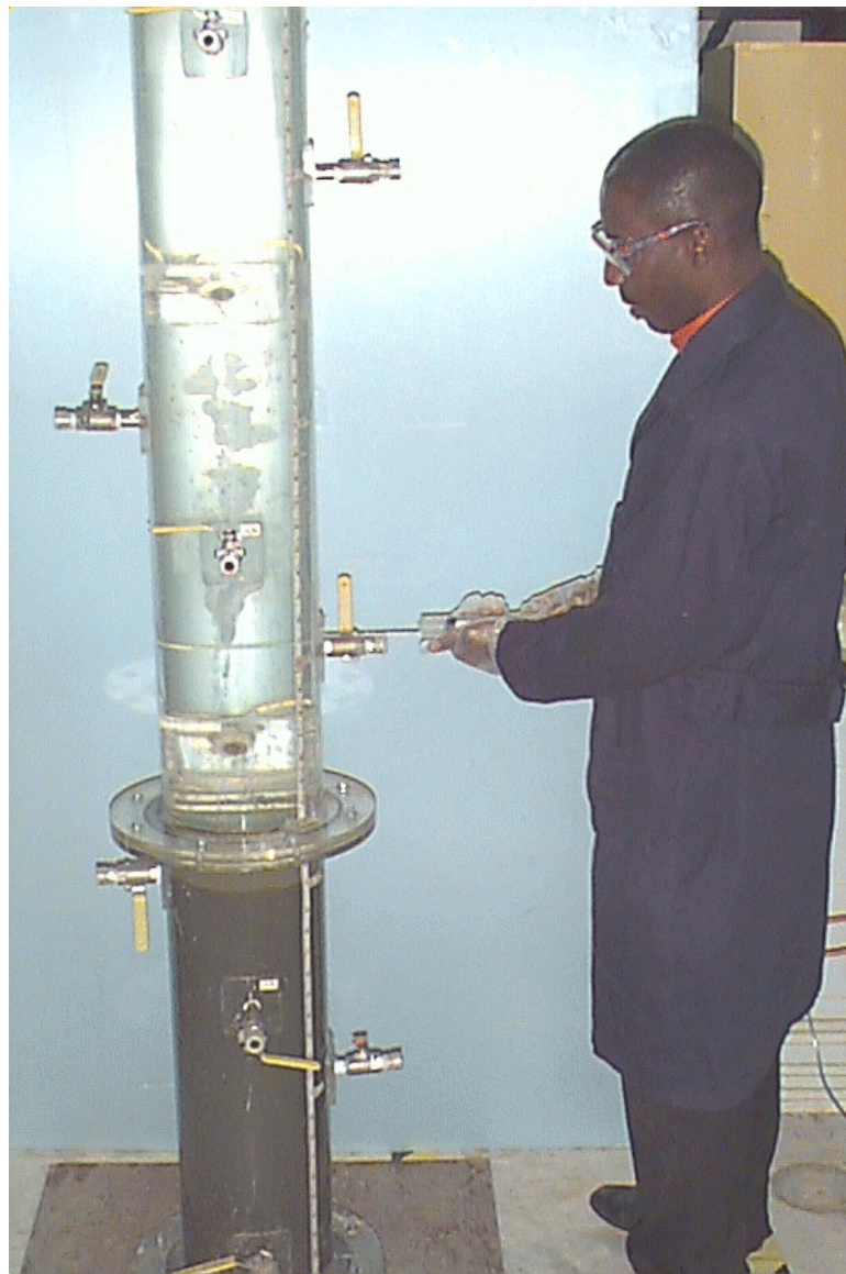
Figure B4. Flocculent test extraction procedure
