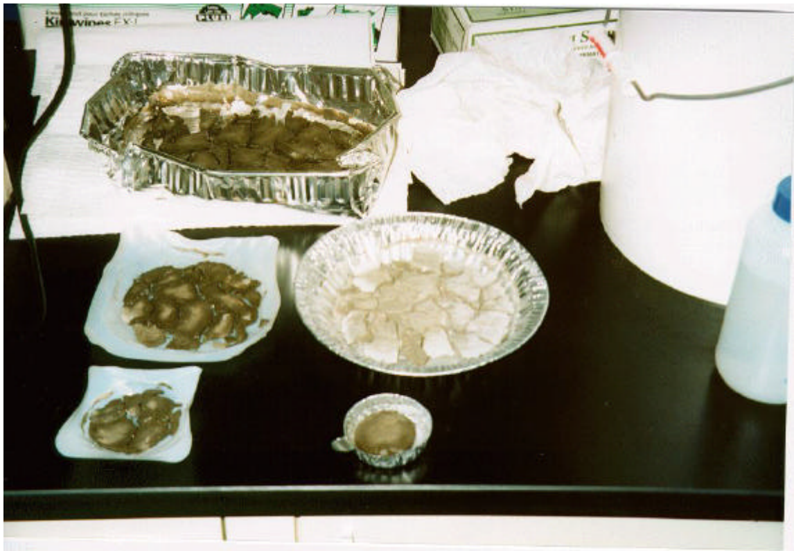
Figure G3. Containers of dredged material used in odor detection test
