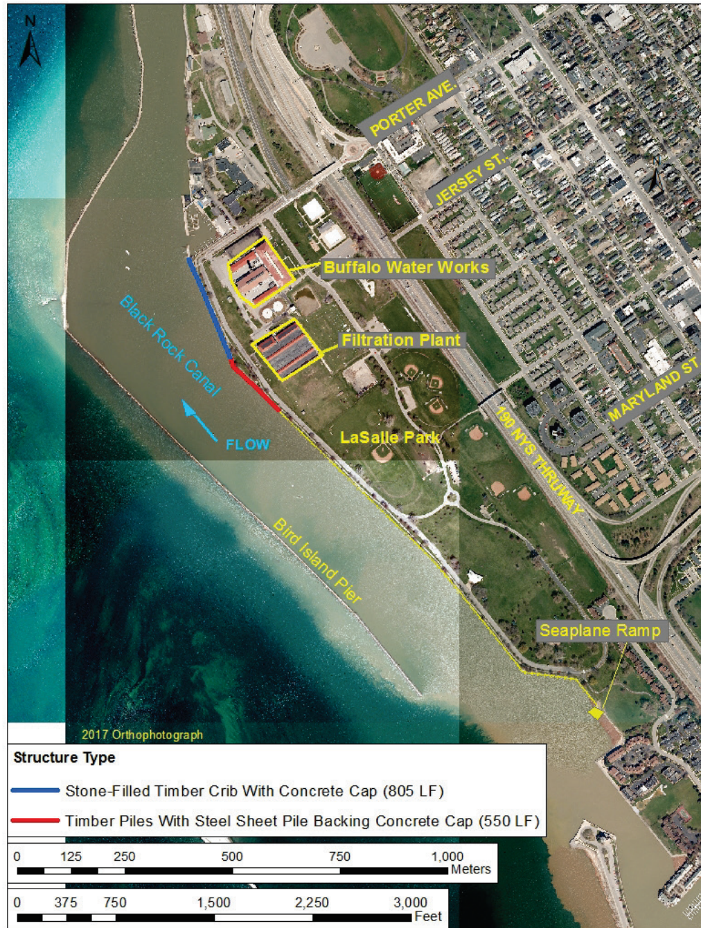
Figure 1-7. LP repair reach (red and blue lines).
