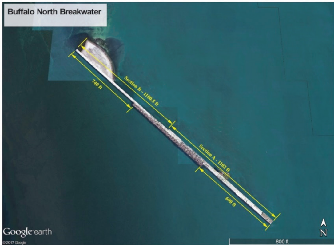
Figure 1-3. The NB structure with four segments
