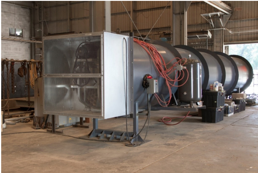
Figure A-3. Cylindrical, open-return, push-down wind tunnel located at GSL in Vicksburg, MS.
