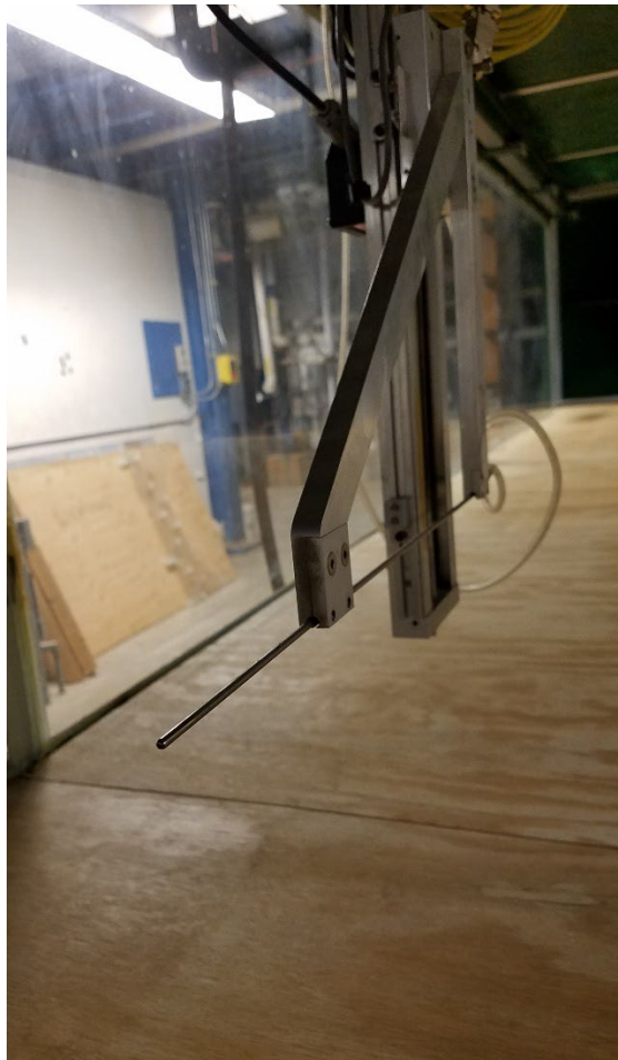
Figure 11. Example Pitot tube secured to the vertical rail of the carriage positioned in-line with the oncoming airflow.
