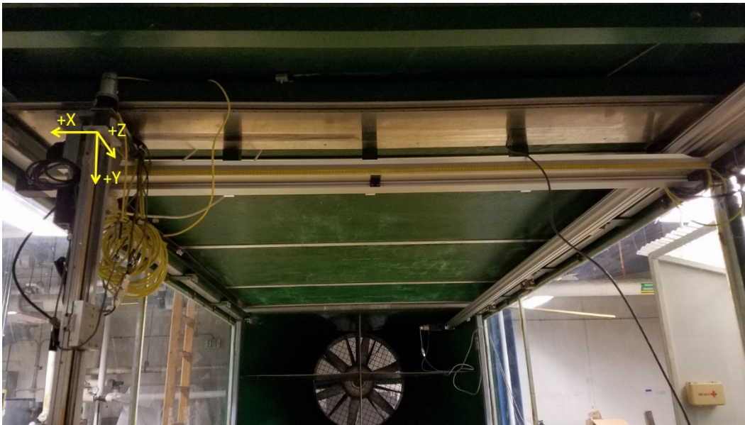
Figure 6. The carriage system within the test section of the CRREL EWT.
