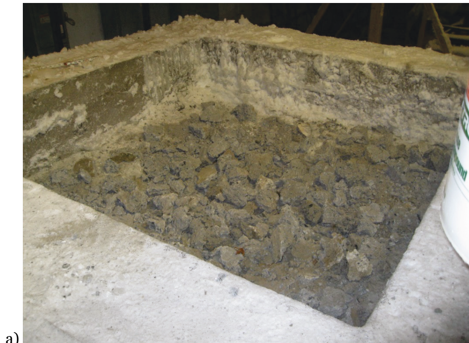
Figure 45. Simulated crater repair performed with debris-reinforced ice: a) concrete debris backfill; b) backfill after introduction of water and, c) after complete freeze-up.
