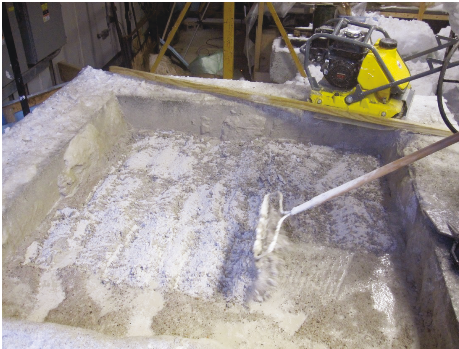
Figure 40. Layer of wetted dry flowable fill being stirred with rake when filling the base of the full scale crater.
