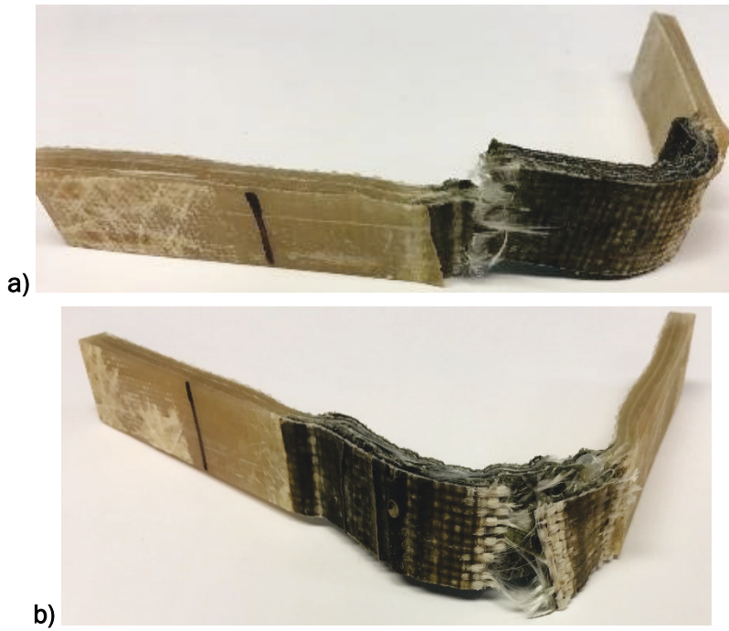
Figure 12. FFM hinge failure modes: a) predominantly, hinges failed at the elastomer-panel junction for the FFM hinges; b) at -40 °F, failure within the hinge was observed.
