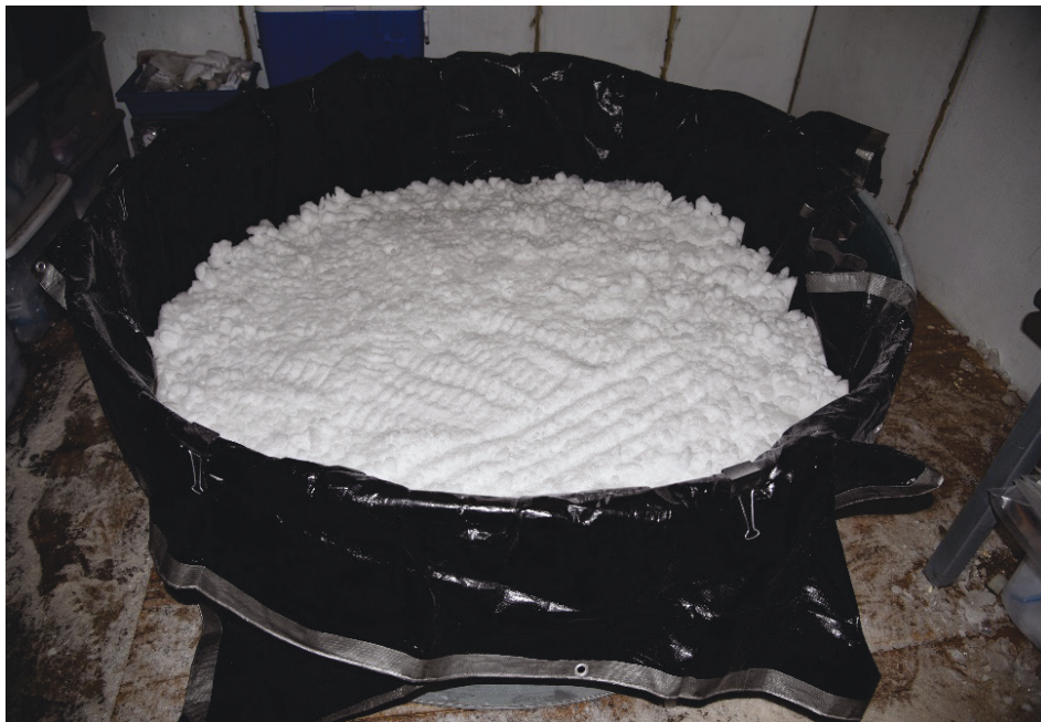
Figure 51. Top surface of dry snow in simulated crater tamped with garden rake.
