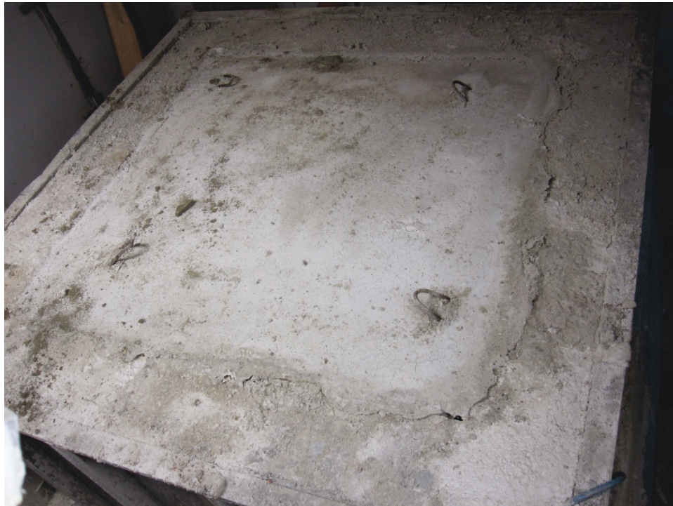
Figure 43. Top surface of mock crater top layer repair with RS concrete after 24-hr since completion.
