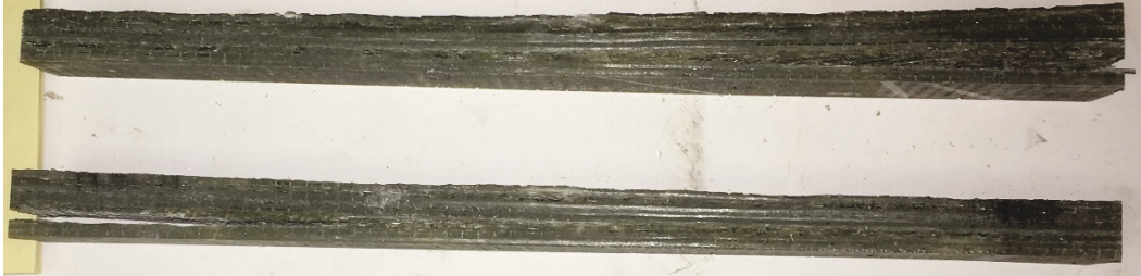
Figure 22. A comparison of the delamination characteristics of the FRP specimens subject to flexural testing: upper specimen was subject to single load-to-failure and shows distinct glass fibers between delaminated layers at the right end; the lower specimen was subject to cyclic flexural testing wherein the glass fibers were worn from between the layers as evident at the left end of the specimen.
