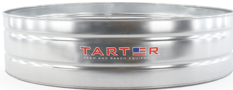
Figure 8. The circular metal form used to simulate a crater for repair with frozen slush materials at -40 °F.
