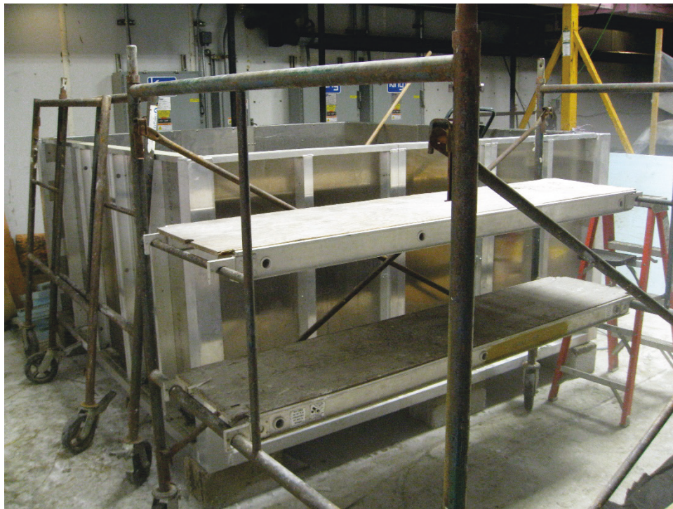
Figure 6. The metal form used to simulate a runway section for full scale mock crater repairs in the cold facilities at ERDC-CRREL.
