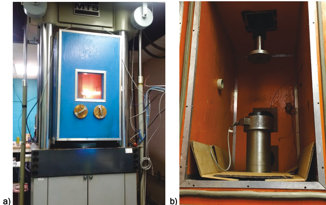
Figure 3. Universal load frame at ERDC-CRREL a) shown with environmental chamber, which allows for temperature control down to -90 °F and b) looking inside environmental chamber to loading platens used for uniaxial compression of cylindrical specimens.
