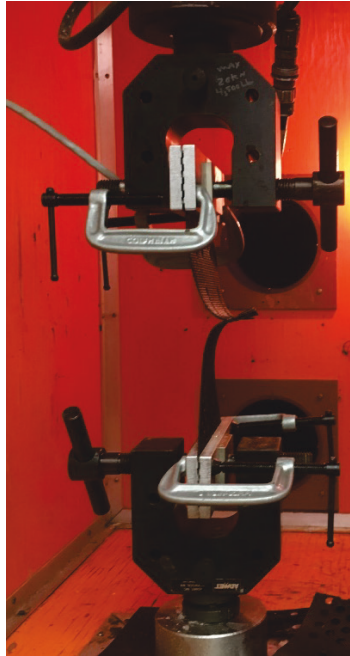
Figure 5. Gripping assembly used to test the geocell specimens.
