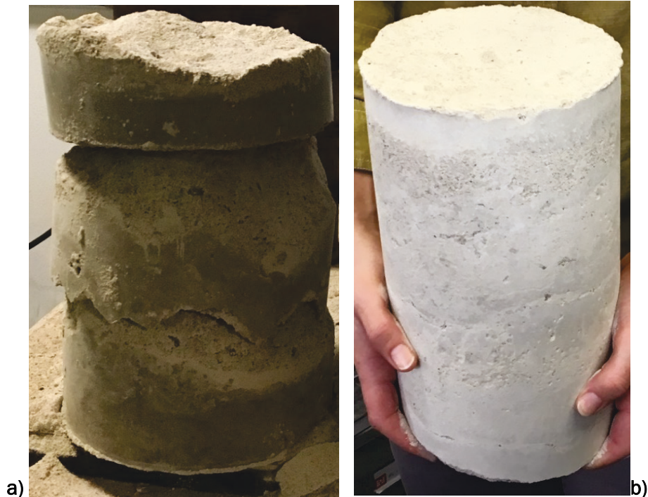
Figure 36. A cylindrical specimen formed using the dry flowable fill technique 0 °F. a) As formed, the lack of cohesion between lifts is seen as the top of the specimen broke and is placed on top. b) After thawing, the specimens were observed to cure, forming a cohesive cylinder.
