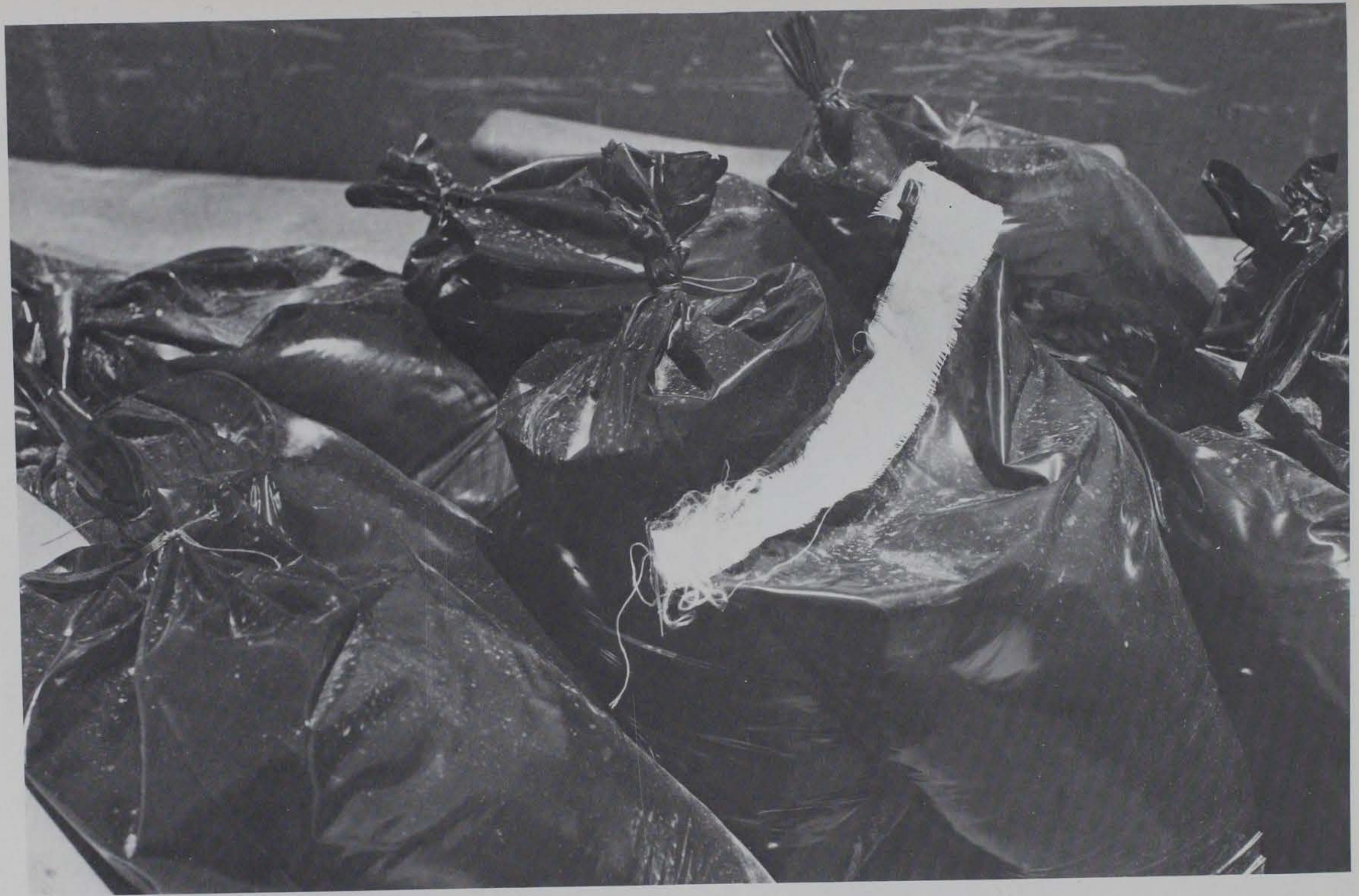
Photograph 11. View showing method used in unsuccessful attempt to sew plastic bags. Also method of tying bags
