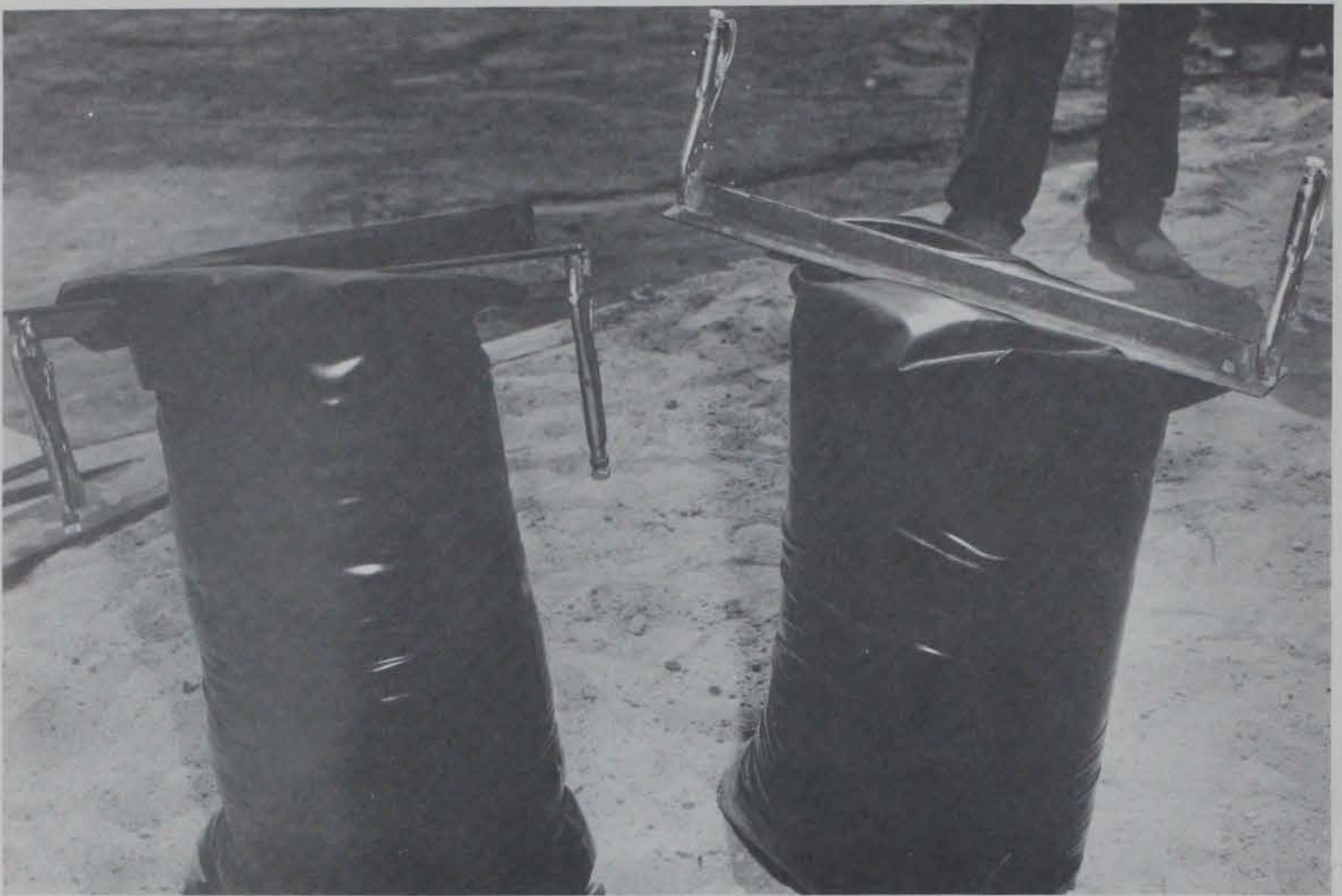
Photograph 9. Two methods used in applying clamping device for heat sealing of plastic bags
