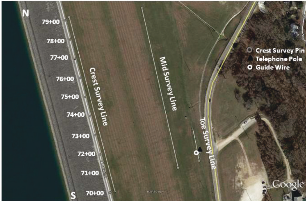
Figure 3. Location of three geophysical survey lines along the downstream embankment. Station 0 of each line aligns with survey pin location 70+00. Google image accessed September 8, 2015.
