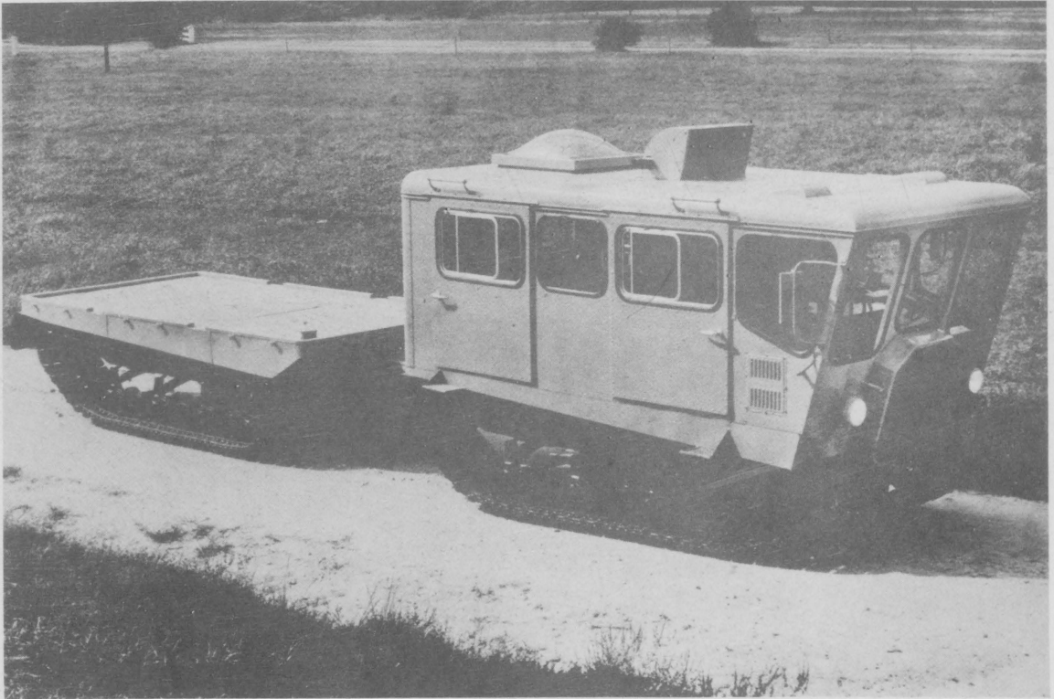
Fig. 3. Articulated, tracked vehicle (polecat) for use as MERS instrument-load vehicle
