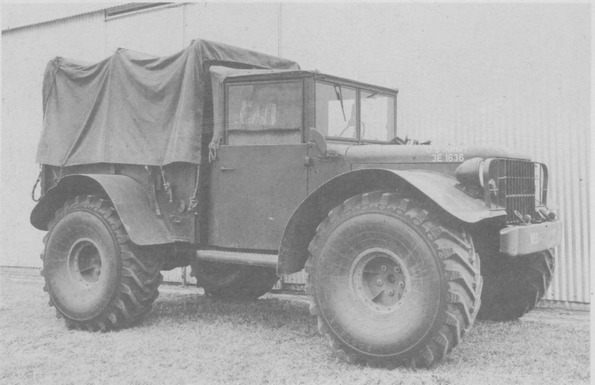
Fig. 2. M37, 3/4-ton cargo truck modified for 46x18-16R high-flotation tires
