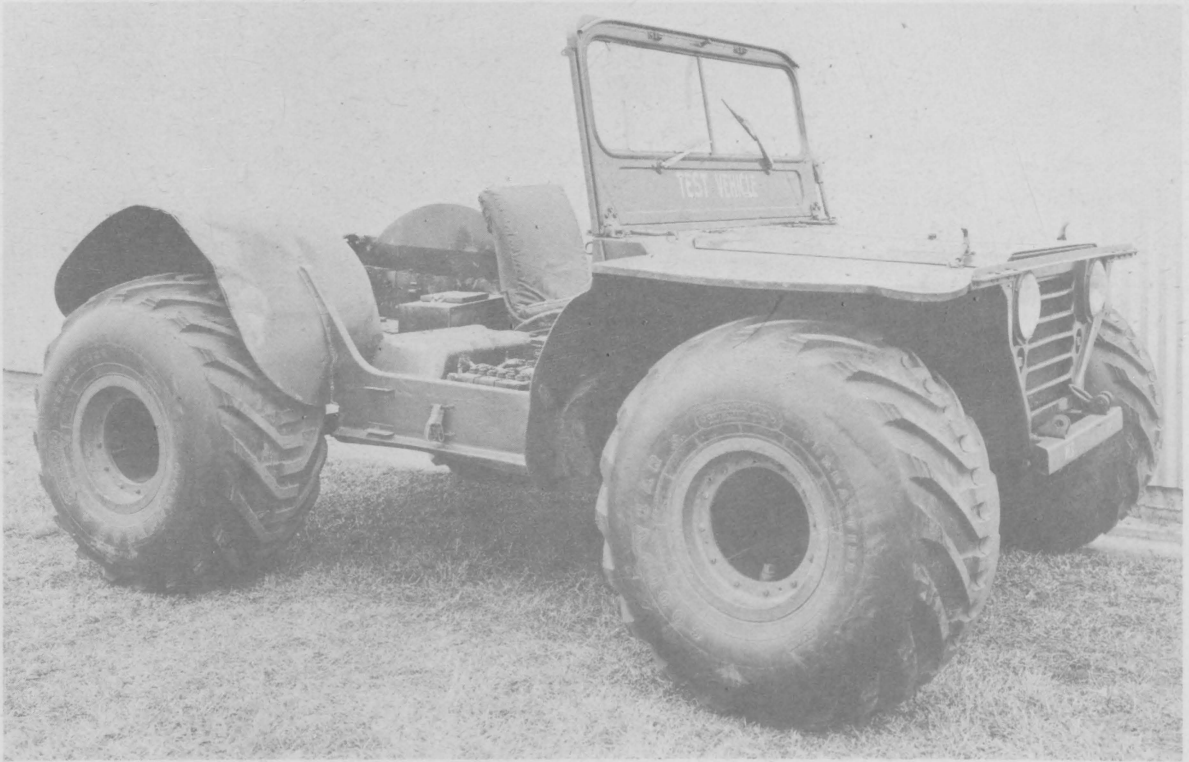
Fig. 1. M151, 1/4-ton utility truck modified for 36x20-14R high-flotation tires
