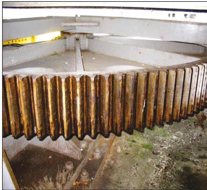
Figure 8. Large gear wheel, showing demanding boundary lubrication operating conditions.
